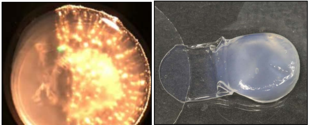
Figure 3: At left is a pig cornea as a flap for a simulated LASIK procedure is being created with the ultrafast beam (a harmonic of the beam can be seen (green color) at center left). The beam is cutting from right to left. At right is the finished flap, approximately 200 \mu\text{m} thick. The clarity of the flap indicates that there were no thermal effects of the ablation.
