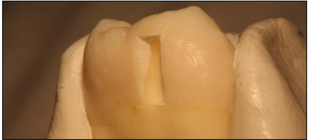
Figure 4: Smart Light™ was used to machine a 1.5 mm x 5 mm trench approximately 1 mm deep in this human tooth. The feature cut through the enamel into the dentin without introducing cracking or thermal damage.
